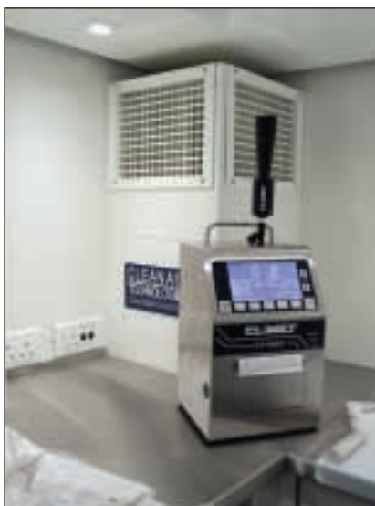
Measuring particle counts in the Arrows Formula 1 trailer
